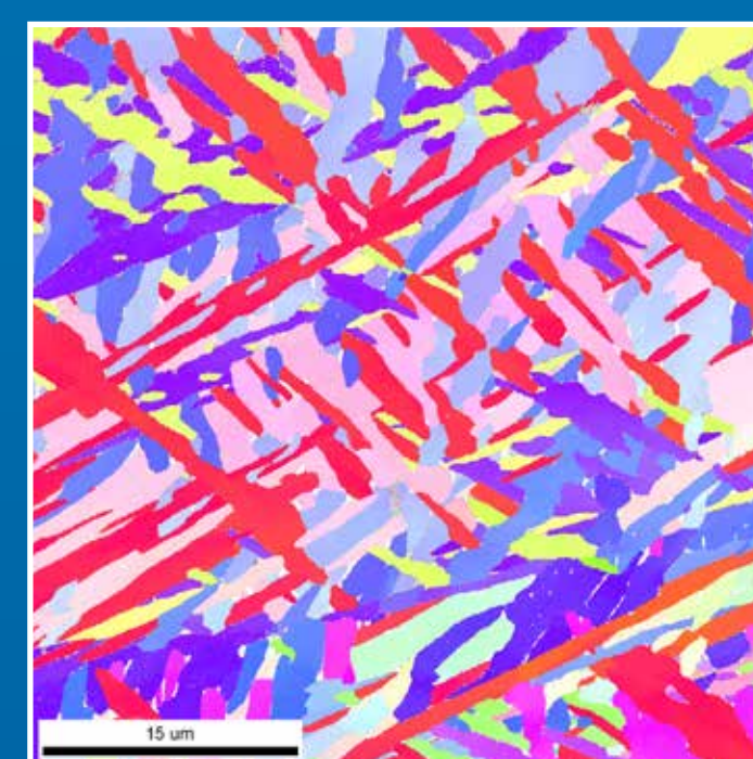
\alpha -Titanium How do you report size for needle-like grains
