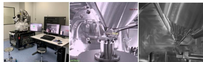
Fig.1 APT preparation by FIB
