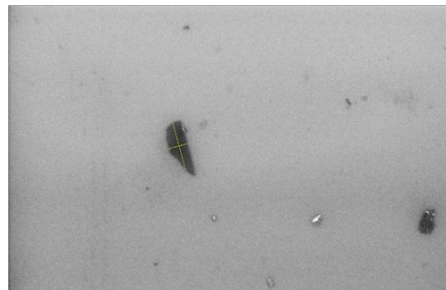
Example SEM image focused on an individual flake. The yellow lines drawn on the flake indicate the lateral size measurements.
