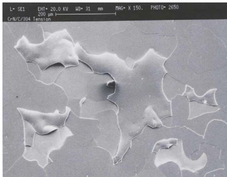
Figure 1. CrN coating on AISI 304 stainless steel with carbon interlayer. Coating spallation induced by differential thermal expansion coefficients when cooling from deposition temperature.
