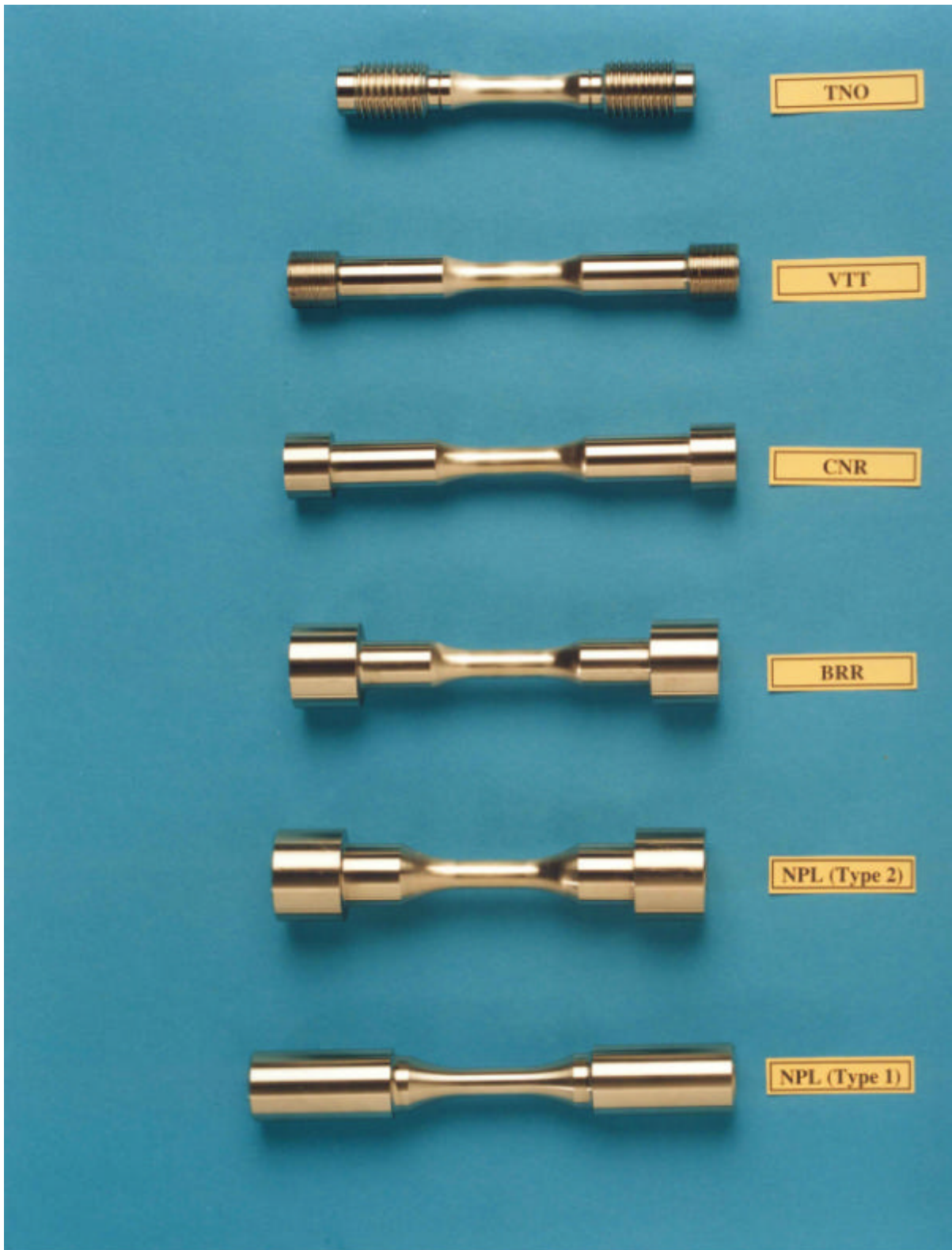
Figure 24. Specimen geometries used in inter-laboratory tests at ambient temperature
